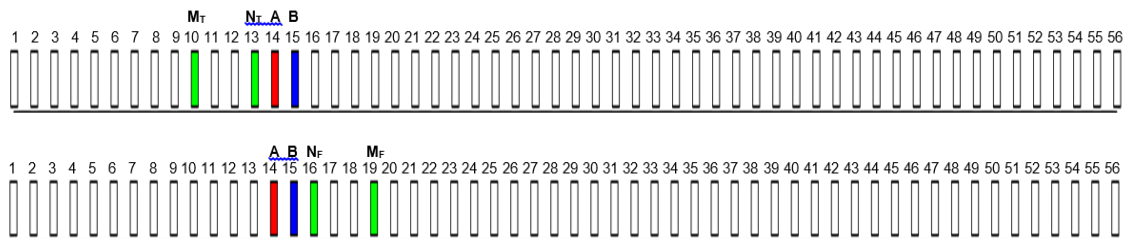
Figure 2.8. The arrangement of an improved dipole–dipole multielectrode array (with the distance of first AB in the position 14 and 15)
